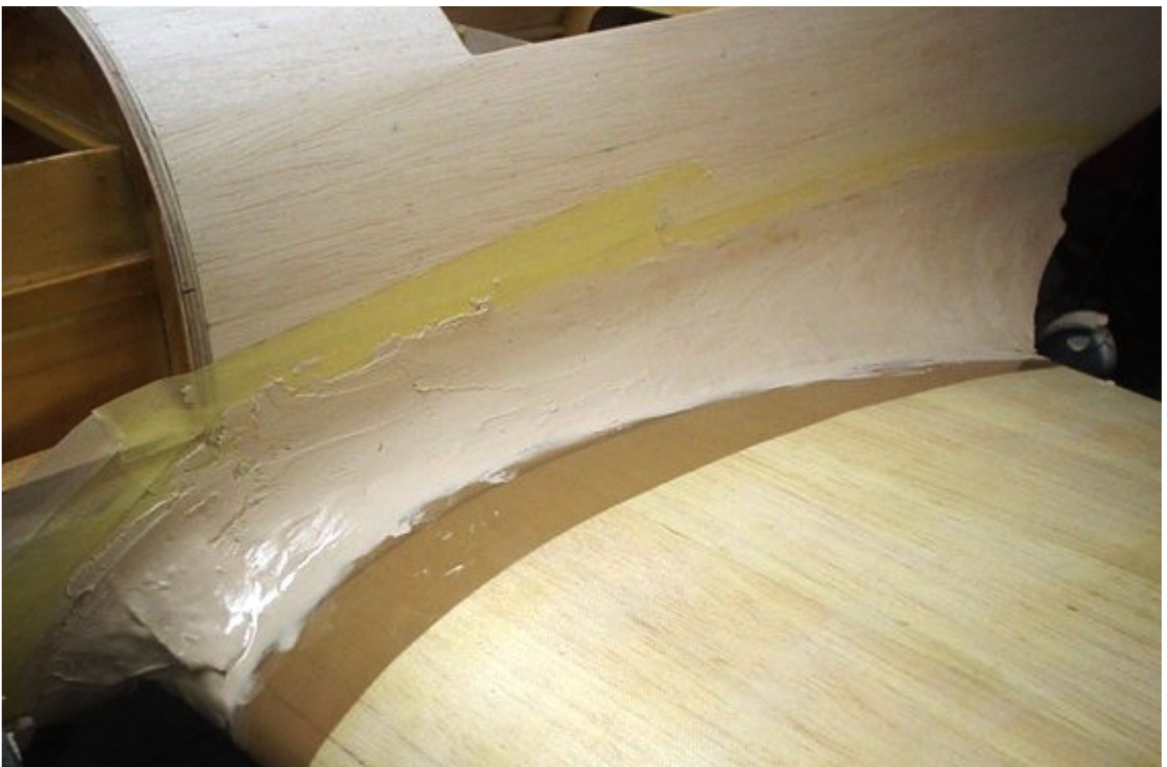
3). Tape top of wing to ensure bog wont stick and then fit wing, bog squeezes out of joint and meets bog applied over rough planking.
