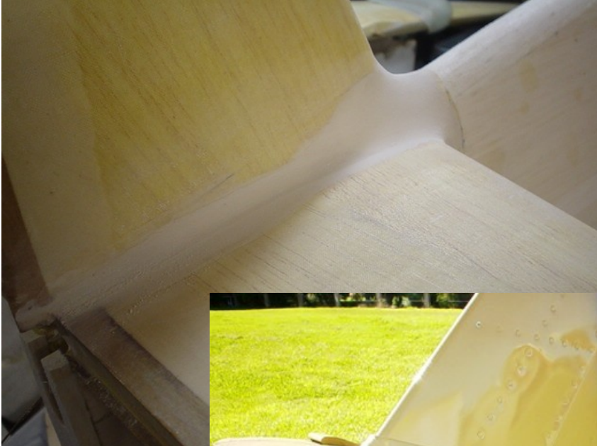
Finished tail fillets.....
